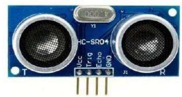
Gambar 2.10 Sensor ultrasonic HC-SR04
